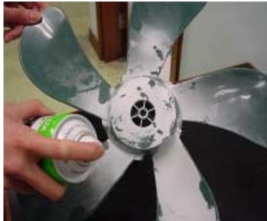
If the profile of the object does not have any distinguished feature there may be requirement to add some reference spheres/ landmarks for further data handling
